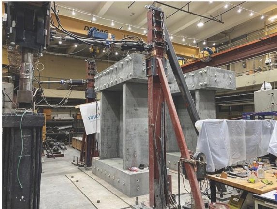
Wall Test Specimens (2) – Phase I
