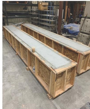
Large Beam Splice Tests (2) #8 Spliced Bars
